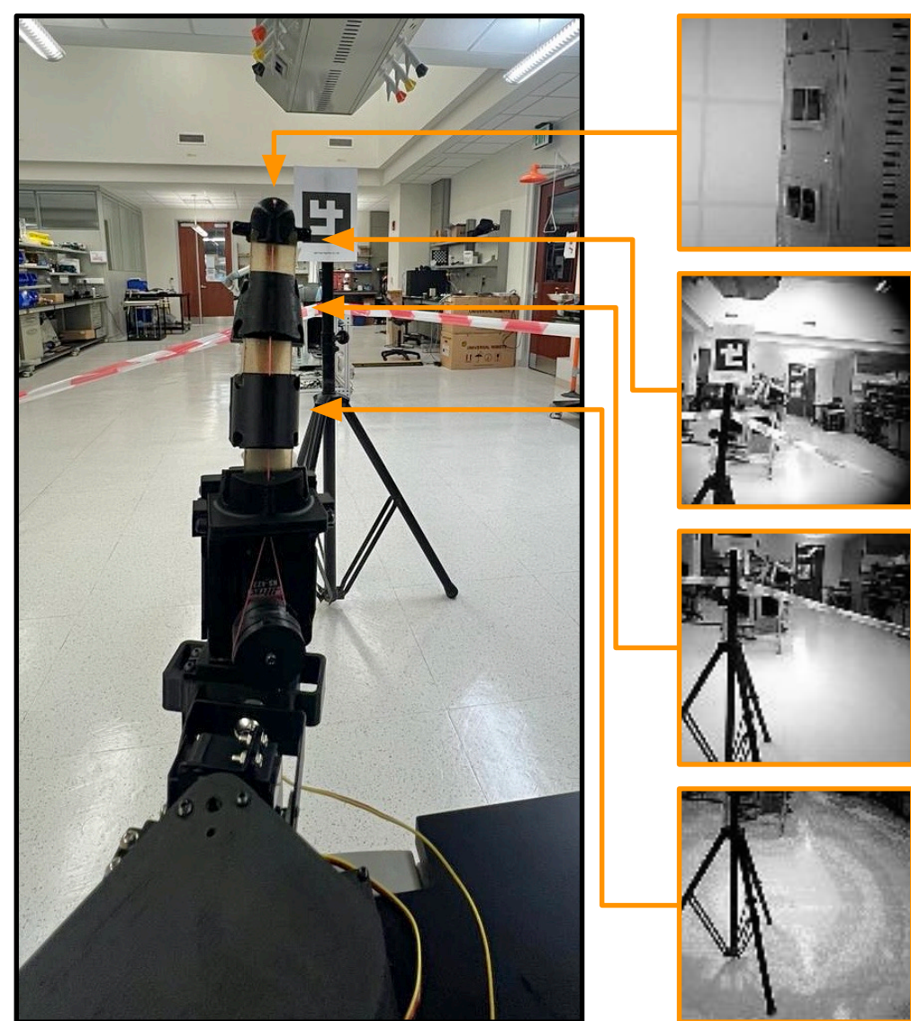
Figure 3: In our experiment, we use the four front-facing cameras and train the robot to move from the central position of the servos to a position where an AprilTag is in sight of one or more of the cameras.
